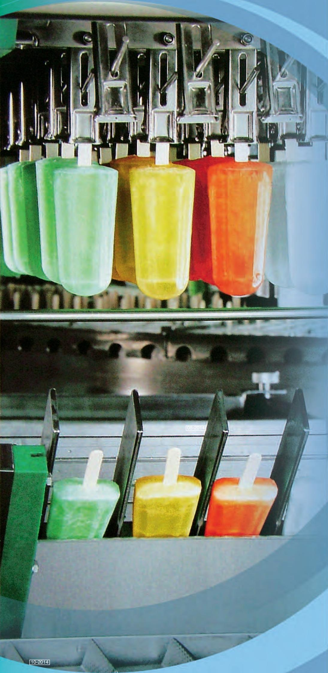
A large industrial machine for producing colorful ice cream bars. The top section shows a tray of molds being filled with green, yellow, red, and orange ice cream. Below, another tray of bars is being processed. The machine has a metallic, precision-engineered appearance.
